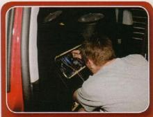
**17.** The back portion of our amp rack was used to house the many Kenwood processors and wiring necessary for the system to work properly. Although hidden from view, these pieces were vital for system operation.
