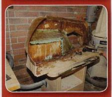
3 & 4. Pop quiz number 2...Can you guess what other material went into the design and fabrication of this system? Fiberglass, lots and lots of fiberglass. The side panels in the rear of the vehicle were too intricate for just wood. Jeff and Dave used fiberglass to make a mold of the area which they will then build off of for the rest of the components.
