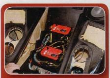
16. You saw our amp rack and how it resembled a staircase as it climbed higher and higher with each amplifier. Because of this we were left with a large space under the amp rack. We thought it was the perfect location for a couple of Optima Redtop batteries and most of the wiring.
