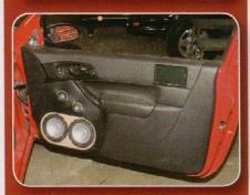
18 - 20. The door panels started out pretty much the same way as our enclosures...with lots of MDF and fiberglass. Once a mold was created it was then wrapped in black vinyl and positioned on the door.
