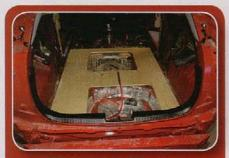
5. With the side panels drying it was necessary to map out the center portion of the system. This is where the amplifiers and processors will ultimately reside. Measurements were taken to determine the precise location of the components before cutting away the MDF.
