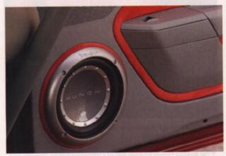
▲ An 800-watt, four-channel Rockford Fosgate amp (PN T8004) powers the main sound stage of two 8-inch RF Punch woofers in the doors, and two RF 5%-inch component speakers mounted in Q-Logic kick panels.
